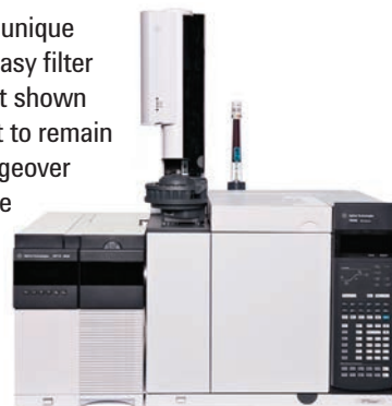
Figure 3. The new bracket integrates the filter with the 7890 GC.
